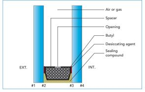
Insulating glazing: components, direction and numbering of sides
