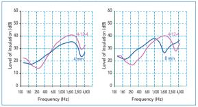
Sound insulation spectrum for 4-12-4 double glazing as compared with single-pane glazings with a thickness of 4 mm and 8 mm
